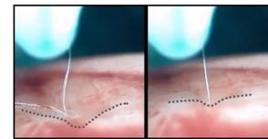
Ex vivo tissue testing (porcine). Without vibration, flexible probes buckle and ~83% of insertion attempts fail; With vibration, insertion failures reduce to ~23%.
