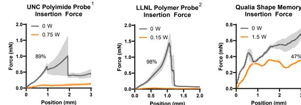
Insertions (and retractions) into agar model (0.5% base with 1.5% top layer), to 2-3 mm depth. NeuralGlider Inserter coupler type and optimized Actuator power settings vary by array. Curves show mean ± s.e.m. for n≥3 insertions for each condition. Insertions with LLNL probe included stiffener.
