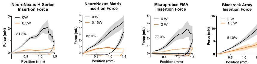
Insertions (and retractions) into agar model (0.5% base with 1.5% top layer), to 1.5 mm depth. NeuralGlider Inserter coupler type and optimized Actuator power settings vary by array. Curves show mean ± s.e.m. for n≥3 insertions for each condition.
